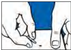
1. Insert receptacle into the drill hole.
